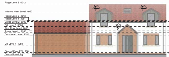
Proposed Front Elevation - Scale - 1 : 100
