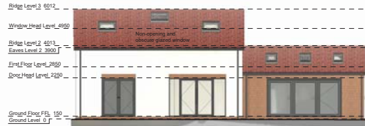
Proposed Rear Elevation - Scale - 1 : 100
