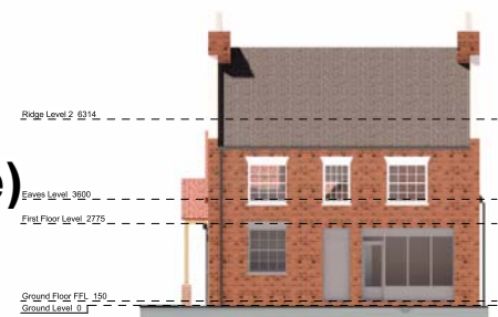
Proposed High Street Elevation - Scale - 1 : 100
