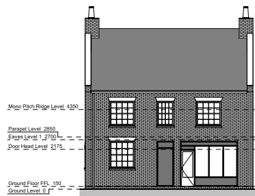
Existing High Street Elevation - Scale - 1 : 100
