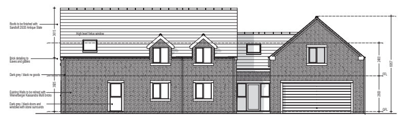
PROPOSED FRONT ~ NORTH ~ ELEVATION 1:100
