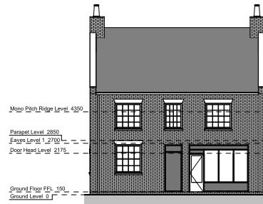
Existing High Street Elevation - Scale - 1 : 100
