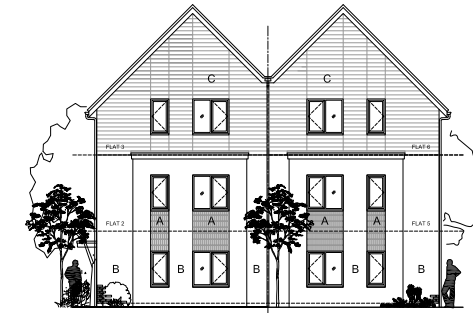
HOUSE TYPE A 3nr 1b2p APARTMENTS FRONT ELEVATION A: STACK BONDED BRICKS B: BRICKWORK C: CLADDING D: INTERLOCKING CONCRETE ROOF TILE
